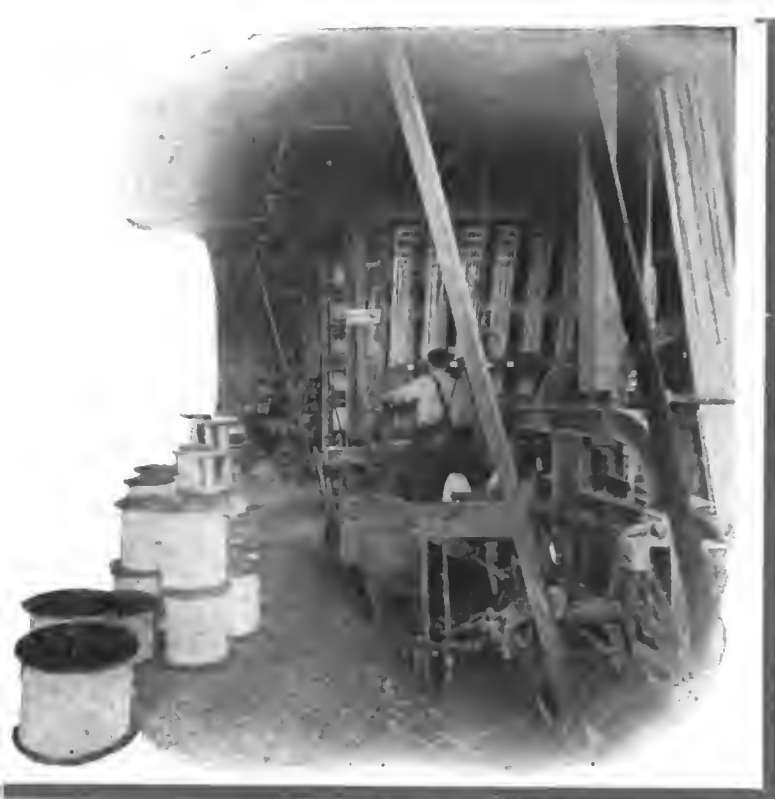
RAYBESTOS is—and always has been—made of the highest quality of long fibre asbestos spun in the form of yarn around wire.
